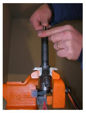
Push nozzle down and untie nut completely. If necessary clean rest of carbon with break cleaner.
