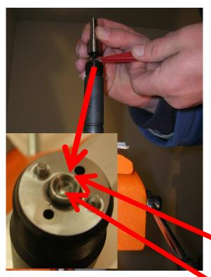
Take the tweezers and hold injector sleeve in place, remove nozzle and needle together from the injector body. Sometimes happens that sleeve and distance bla get loose
