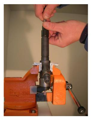
Grease the threats of injector body and nut with Vaseline, push nozzle down like by disassemble and hand tie nut (still push nozzle down, needle is preloaded of injector spring)
