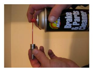
Place nozzle back on injector body, line up the position pins (pins are 1mm eccentrically) Clean nozzle body first with break cleaner, if you have an ultrasonic cleaner (jewelry cleaner) by hand → much better and lay nozzle body by side where it doesn't get contaminated with dirt or particles. Clean needle as second and assemble back into nozzle.
